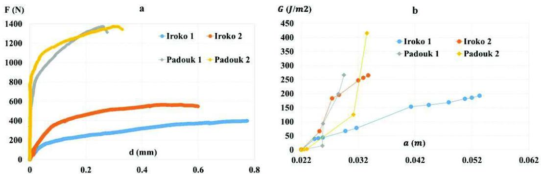
Figure 2. Force-displacement curves (a) and critical energy release rate- crack length curves (b)
