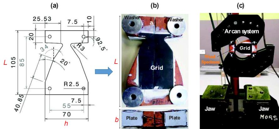
Figure 1. dimensions of specimen (a); side of crack initiation and face with grid (b), experimental device (c)
