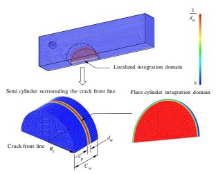
Fig. 6: Integral cylindrical plate domain around the crack tip
